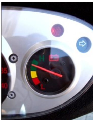
Battery Charge Meter
