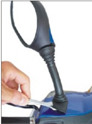
Installing a mirror or adjusting
